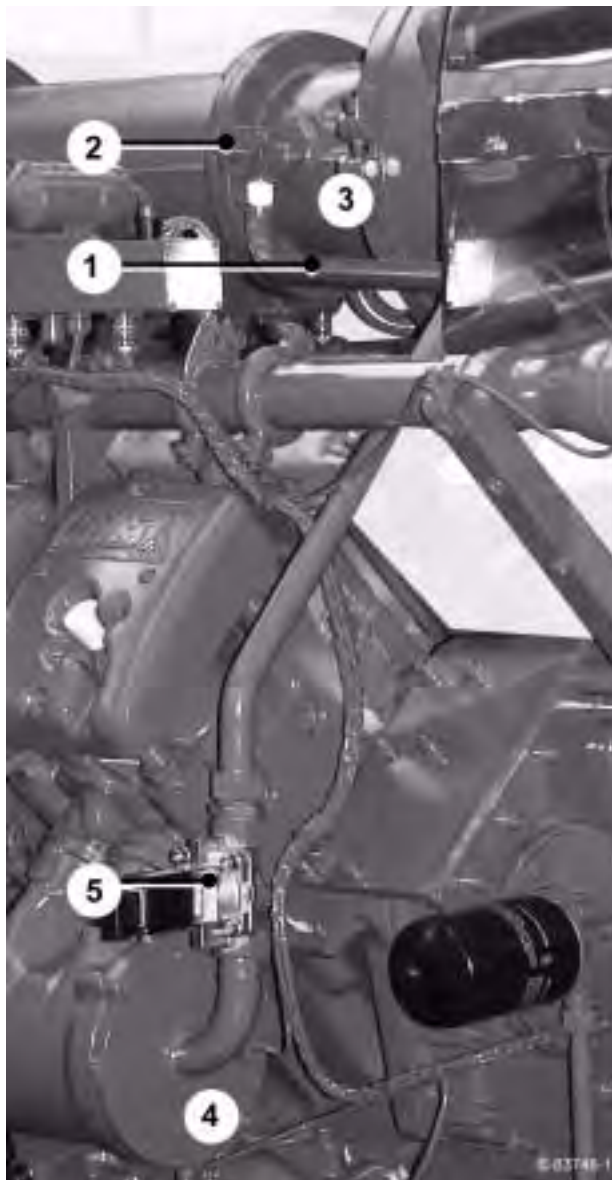
A 2-19 Compressor bypass (two-gas operation)
